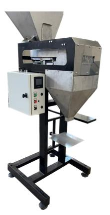
or through various types of automatic loading systems and by selecting the dedicated recipe, previously saved via the intuitive touchscreen panel on which all the management parameters are available, it will be possible to weigh and fill preformed bags, jars or boxes.
